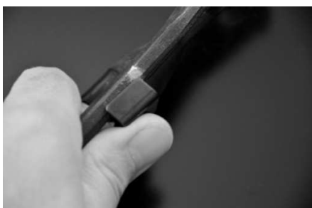
5. Latch clamping lever half way on the lower handle
