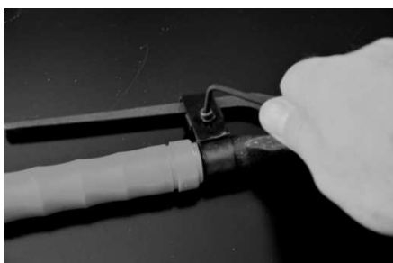
6. Tighten the screw on clamping lever DO NOT OVERTIGHTEN THE SCREW
